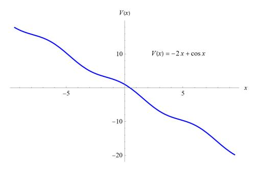
The graph of V(x) versus x is to be thought of as a two-dimensional rollercoaster. A particle placed anywhere on the curve will roll indefinitely to the right because the slope is never zero; in other words, there are no equilibrium points.
